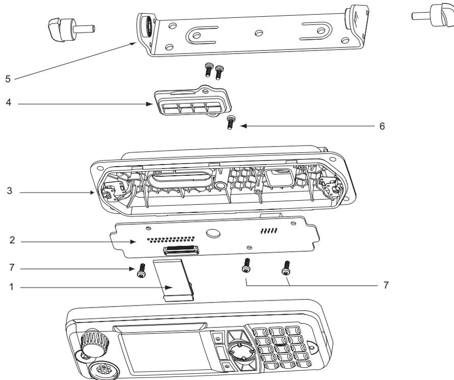
**Figure 6-56** Remote Mount Enhanced Control Head – Exploded View
